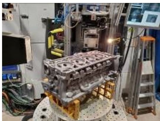
Figure 3. Neutron measurement of the cylinder head sample with SALSA at ILL.
