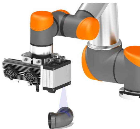
Figure 1. 3D scanner mounted on the X-Raybot.
